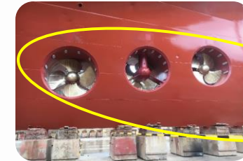
3x Bow Tunnel Thrusters (oilfieldtechnology, atzmartec)
